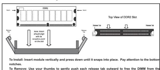
Figure 5-3. DIMM Installation
